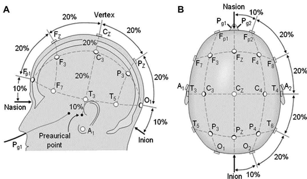
**Figure 3** International 10/20 system for electrodes. (A) Lateral view of the electrodes montage. (B) Superior view of the electrodes montage.
